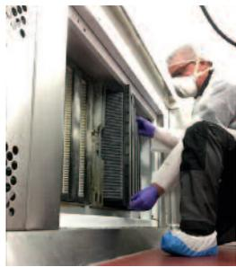
Daily visual checks such as checking for panel damage and failed lighting are a start point and can be done by the operator, who probably knows the unit better than anyone.
