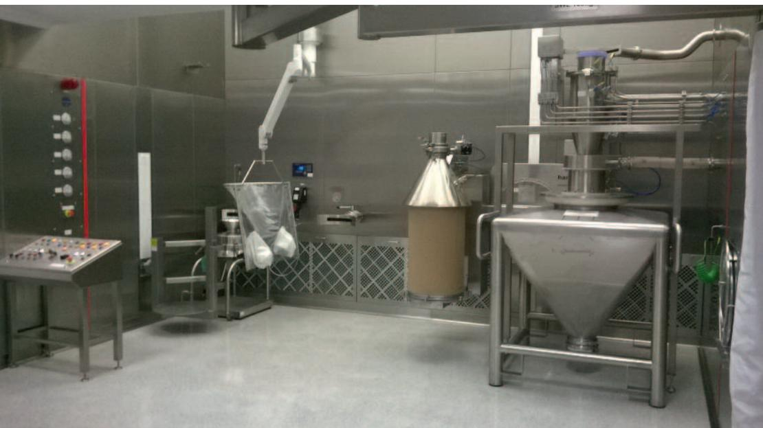
Hosokawa engineers designed a bespoke, 5m wide, recirculation, dispensing downflow booth suitable for the handling of OEB3 compounds with a time-weighted average less for process operator level (OEL) less than  $0.100\text{mg}/\text{m}^3$  ( $<10\mu\text{g}/\text{m}^3$ ) with the addition of a high containment barrier screen.
