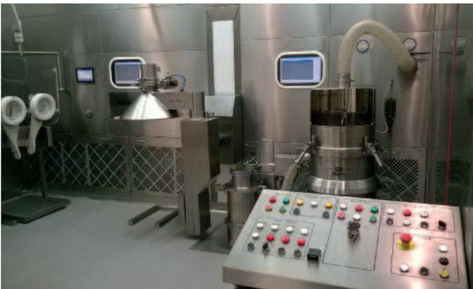
The requirement was for a dispensary downflow booth designed to support dispensing, weighing, delumping and material handling of Level III active pharmaceutical compounds with containment systems to provide consistent operator protection from hazardous airborne particles.
