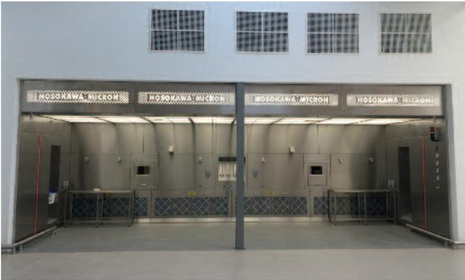
The scope of supply was for one booth suitable for the handling of powders and another, smaller booth suitable for handling solvents.
